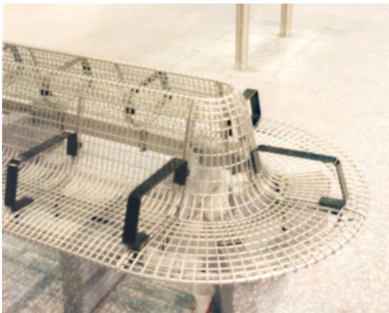
*Electropolished lattice wire structure in stainless steel for the North Greenwich Station bench seats.*
