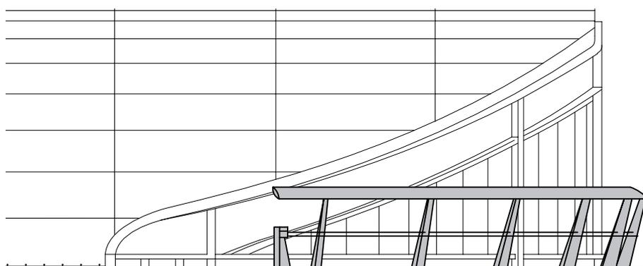
*Both leaning pads and cable barriers are supported on inclined 'T' section stanchions made from matching 1.4401 stainless steels.*
