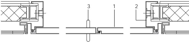
*Brake pressed panels use satin finished grade 1.4432 (X2CrNiMo17-12-3), in thicknesses of 2 and 3 mm. The secret fix cladding and doors are flush fitted. Doors have hidden hinge pivots and are 1 hour fire resistance rated through the use of panels which are backed by a quilt of mineral wool.*
