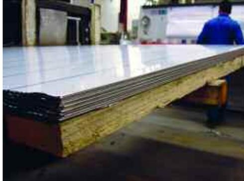
*Stainless steel sheet can be supplied with a protective plastic coating.*
