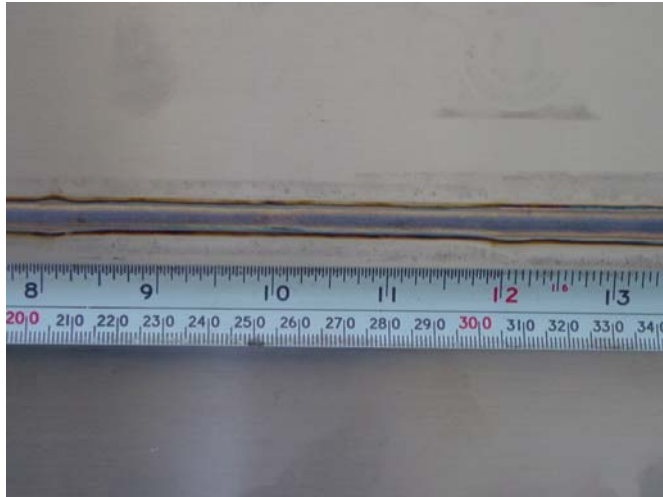
Fig 4. Heat tint on the cap of a TIG weld
