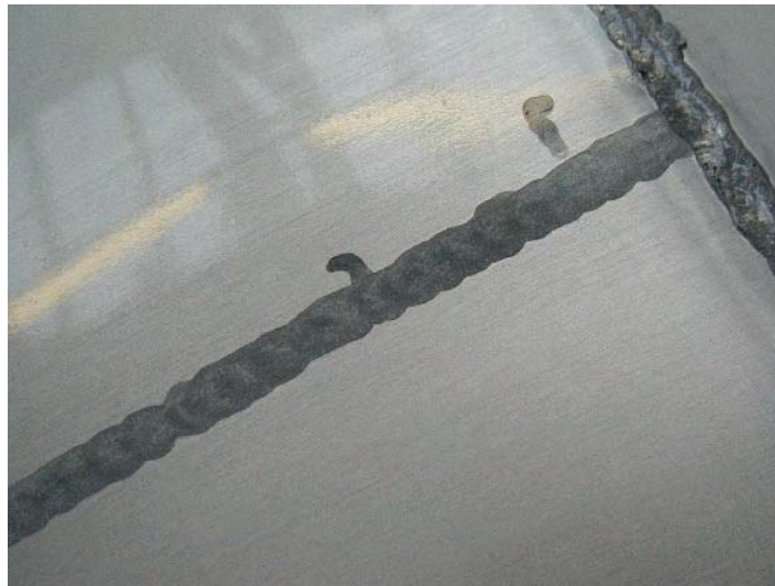
Fig. 8. Surface finish changed by pickling (Courtesy of Stainless Restoration Ltd)
