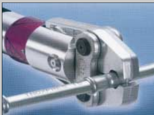
A pressfitting tool clamping an Inoxpres fitting (Photo courtesy of Lancashire Fittings)
