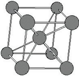
This is called a Body Centred Cubic (BCC) structure for fairly obvious reasons. There is an atom at each corner of a cube and one in the middle. The arrangement of atoms is called a lattice. The atoms of carbon are smaller and have to fit in as best they can within the structure. In iron and steel this structure is also called ferritic.
